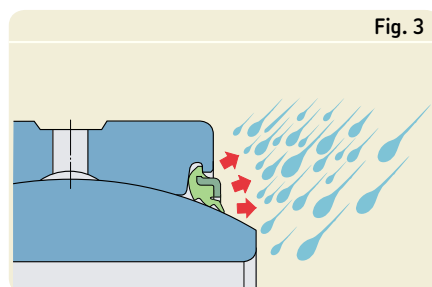
Three seal lips keep contaminants out
