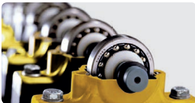
Emcor grease test rig
