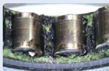
Lubricant degradation caused by electrical discharge currents
