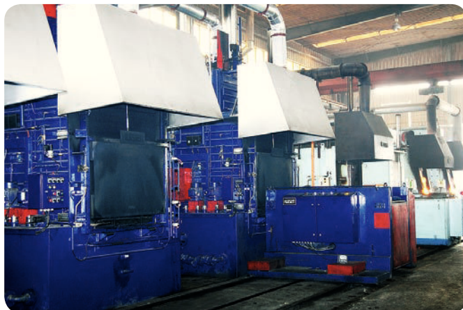
Furnaces for heat treatment process
