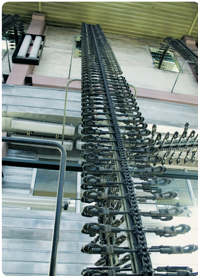
SKF Hollow Pin Chains used on a newspaper conveyor
