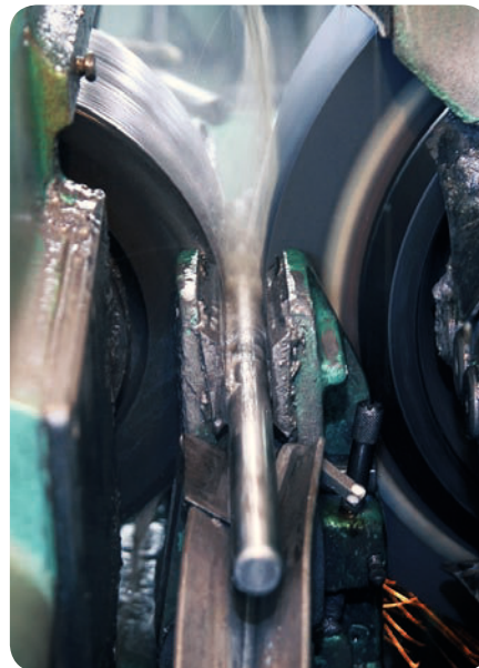
Pins are precision ground to enhance wear resistance and increase chain service life
