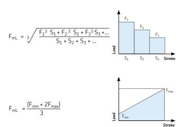
$F_{mL}$  = constant mean load for lifetime calculation in N
