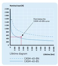
In this example, the CASM-40-BN is the smallest possible linear unit.
