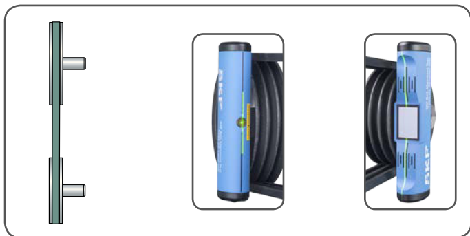
Figure 9 Pulleys perfectly aligned
