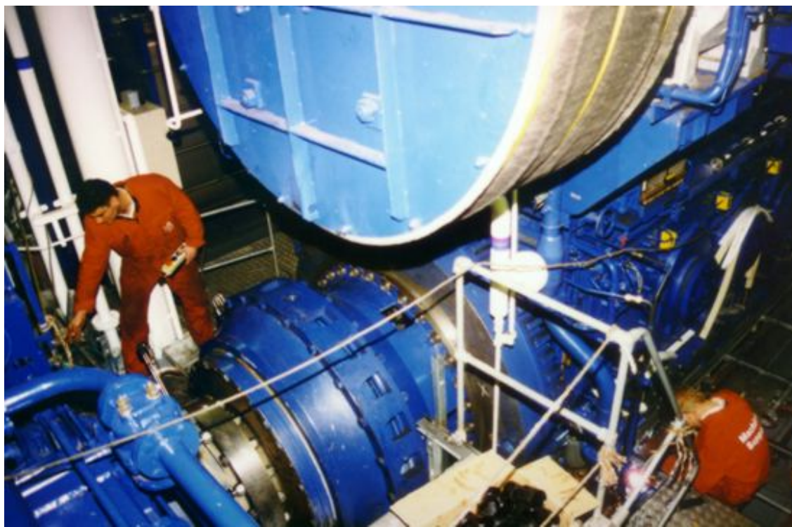
Figure 5.1.3.1 Alignment and chocking of components are typical Machine Support activities.
