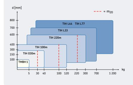
The comprehensive range of SKF Induction Heaters is suitable for most bearing heating applications. The chart gives general information on choosing an induction heater for bearing heating applications.<sup>3</sup>
